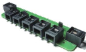
I have built an RJ12 box, which optionally also contains the two diodes for the pseudo-GND (see [RailSync-Current-Limiter-Device \(RSCLD\) RSCLD Urversion](#)) and a resistor like [here](#). The pseudo-GND can be connected via a jumper. I have not currently fitted the resistor contained there. An assembled resistor can be bridged with a jumper if required. The pseudo-GND may only be present once in a RailSync supply section. The circuit fits into the FREDI housing.
