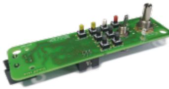
I have adapted the circuit based on the FREDI-1.8C of the [FremoDCC](#) with an SMD type of the ATmega328 and a different voltage regulator, as there were problems with the used LM2936. The [STEC11B03](#) was used as the rotary encoder, the slotted 6mm axis was shortened. Types with high light output (approx. 1000mcd) were used for the LEDs, so that the resistors were changed from 470R to 2.2k.
