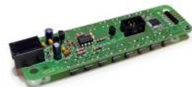
I have realised that not all functions of the PIC-Vers-148 have been implemented in the Arduino sketch, as they are used in [GCA123/GCA50](#). Only the 'Block Sensor' variant is implemented as an input. I have subsequently added an option to the sketch that was also missing in the sensor function. This is the 'Active High' option, which I use for [switch control](#) with Rocrail. For my application, both LocoIO keypad variants are now equivalent.
