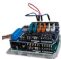
In parallel to the [SPROG3](#), a command station was built on the basis of the Arduino Uno. This also requires a [MotorShield](#). The [wiring](#) and the [integration](#) will be found at rocrail.
