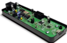
The LocoBuffer-ProMini was developed by combining the circuit design of the [LNShield-ISO](#), the Arduino-Pro-Mini and a USB-to-serial converter. The module realises a galvanic isolation between PC and LocoNet via the optocouplers. As with the LNShield, Tx can be configured on D6 or D7 via a jumper or wire bridge. Rx is on D8. The **15mA LocoNet current source** (pull-up) can be activated via jumper **JP4**.
